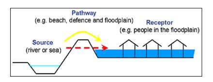
Figure 1: Source-Pathway-Receptor Model (adapted from <u>www.floodsite.net</u>)
